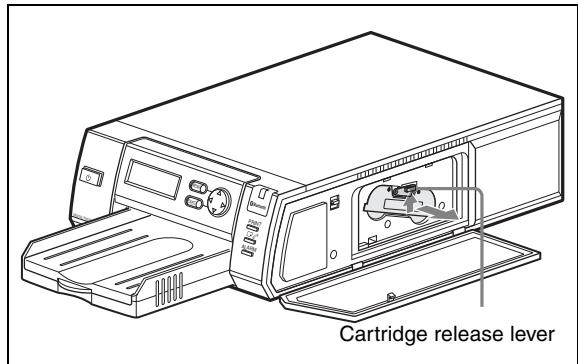
The cartridge is released, allowing you to pull it out.
